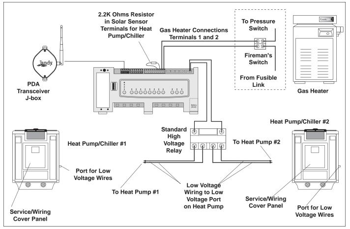
Figure 16. Heater and Heat Pump/Chiller Wiring
